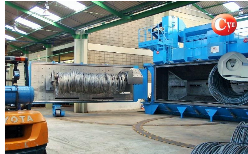
Mechanical pre-treatment Shoot blaster for wire rod coils – source Fa. CYM
