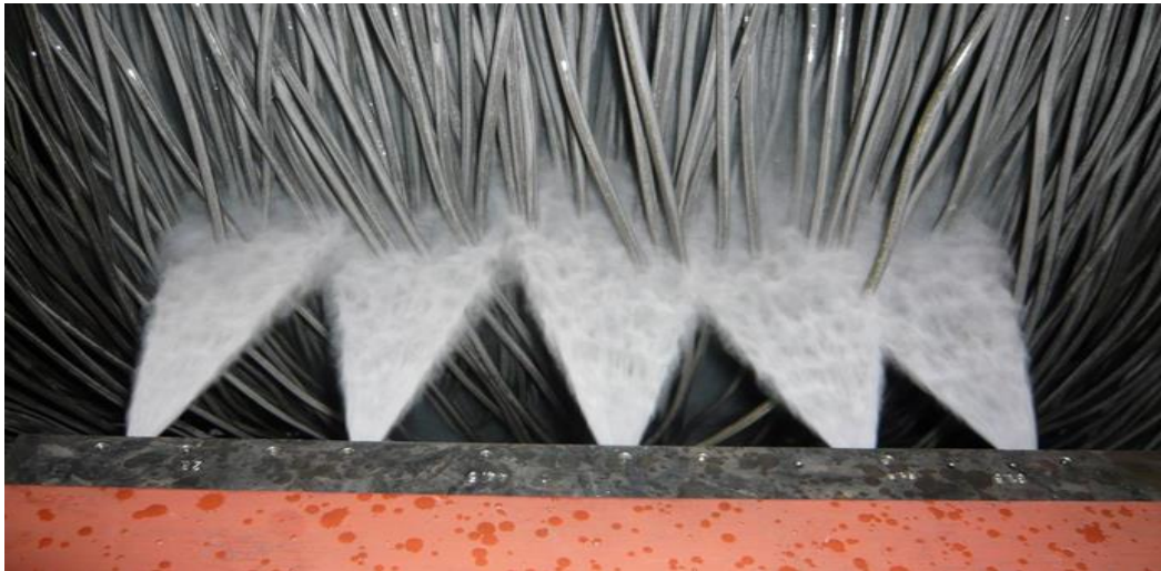
High pressure descaler – Pilot trials – source: BFI, stahl&eisen
