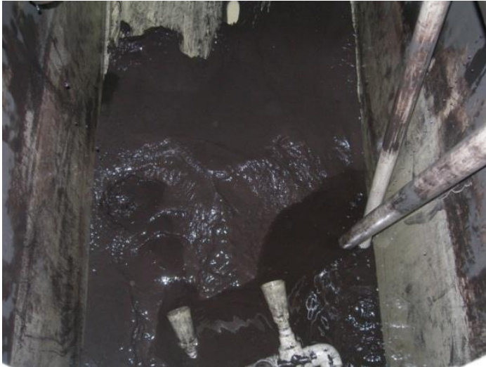
Backwash / Cleaning with solids discharged from ASRA vessel as an slurry with approximately 30% wt/v solids.
