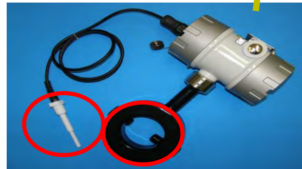
Body: EFTE coated steel Temp sensor: PTFE
