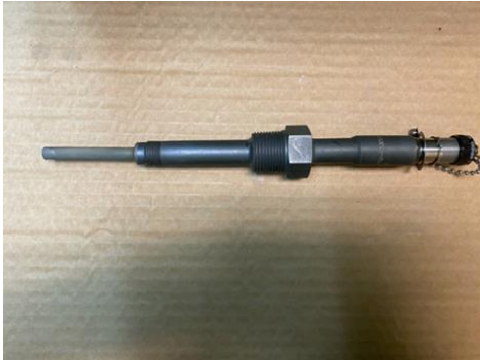
Figure 5: Cylindrical carbon steel corrosion probe with a span of 127 mkm
