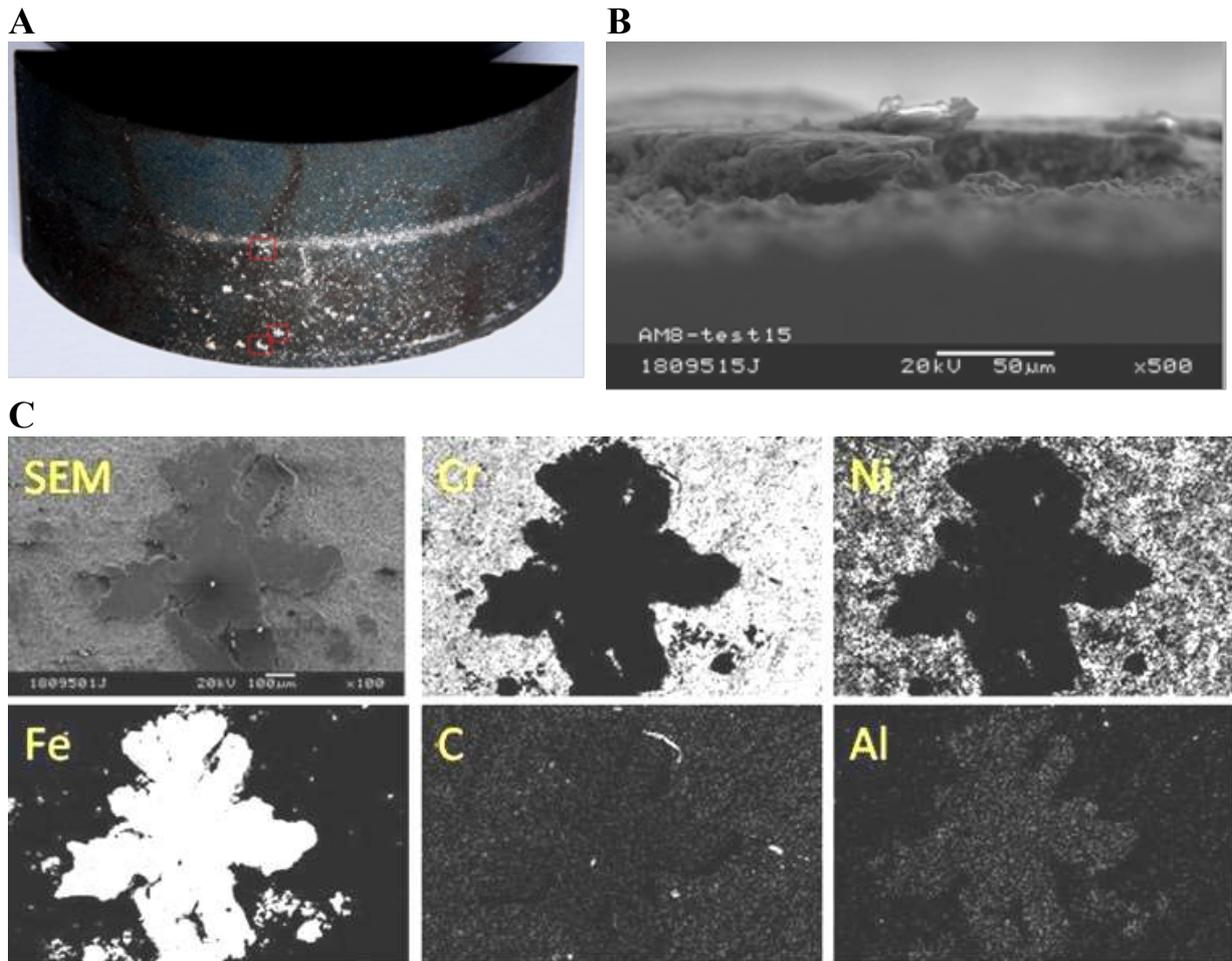
Fig. 8: (A) Photo of the Cr<sub>3</sub>C<sub>2</sub>-NiCr roll showing pickups; (B) SEM lateral view of a pickup; (C) SEM-EDX mapping around a pickup (top view).
