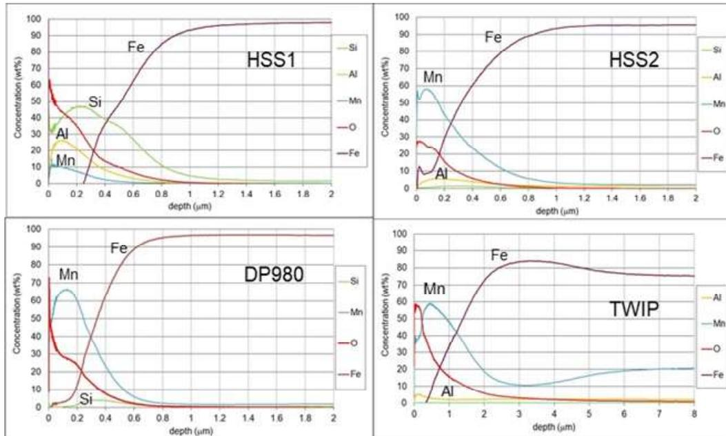
Fig. 3: GDOES quantitative depth profiles of the steel samples after oxidation at 900°C in 7%H<sub>2</sub>-N<sub>2</sub> with DP of -40°C.
