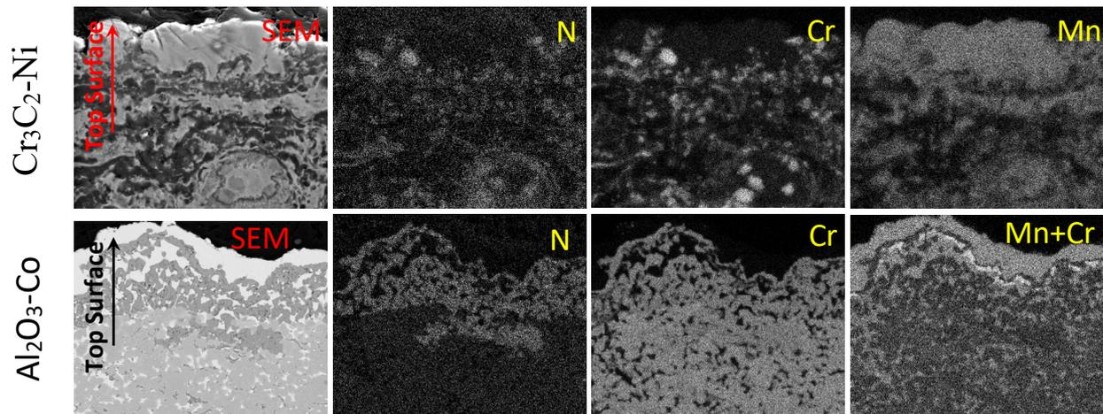
Fig. 6: SEM mapping shows nitriding and Mn oxide sticking and diffusion inside the coating (900°C; DP=-30°C)
