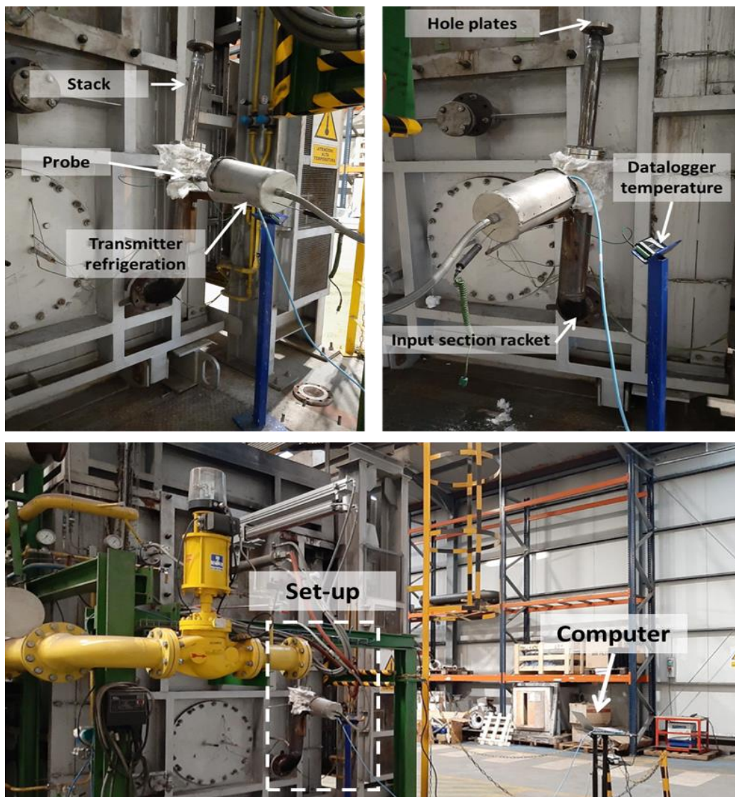
Figure 4: Industrial experiment setup for corrosion probes at ArcelorMittal Gijon plant
