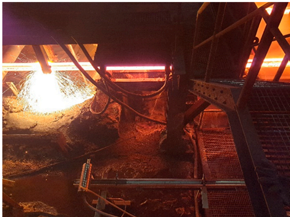
Figure 1. Laser vibrometer mounted on rail to measure strand vibrations along ESF billet caster.
