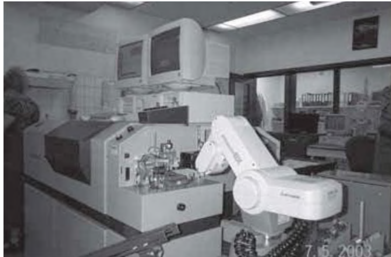
Equipment used for pre-industrial test – 2 burns for steel composition (3 min); after 3 additional burns, determination of cleanliness index (+3 min)
