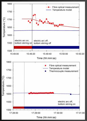
Without bottom stirring temperature homogenisation approx. 50 seconds after powering off the electric arc
