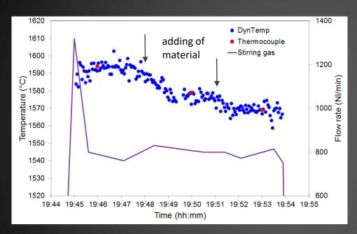
Liquid steel temperature evolution during gas stirring using an adapted stirring lance as measured by fibre optical and thermocouple measurements.
