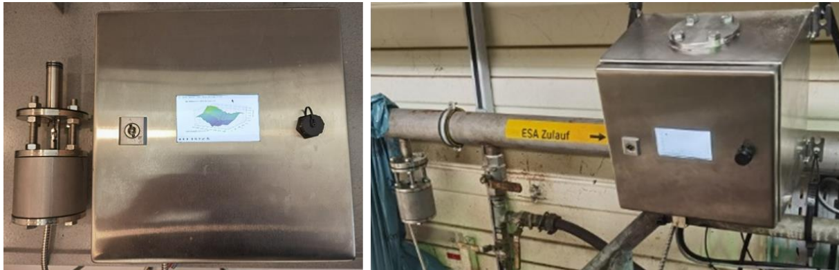
Figure 10 NIR-Measurement device set-up and operational installation at ESP emulsion feed
