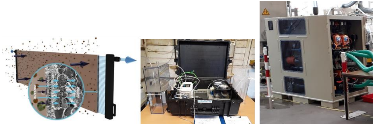
Figure 3 Ceramic flat sheet module (left) - lab MCDI (middle) - field trial MCDI (right)
