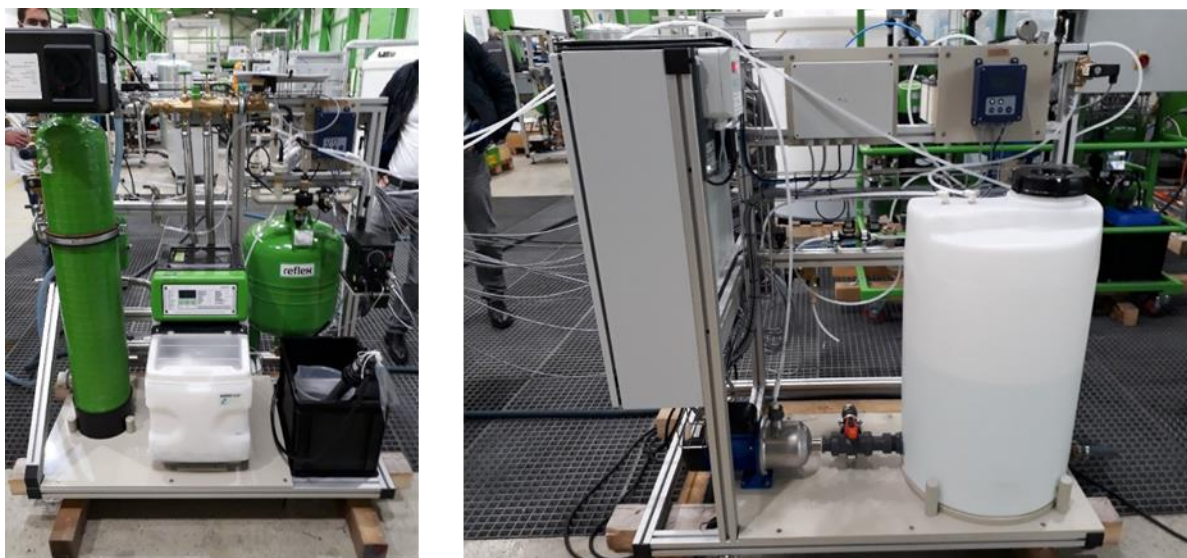
Figure 5 Pre-Treatment unit (left) and MCDI plant (right) at BFI
