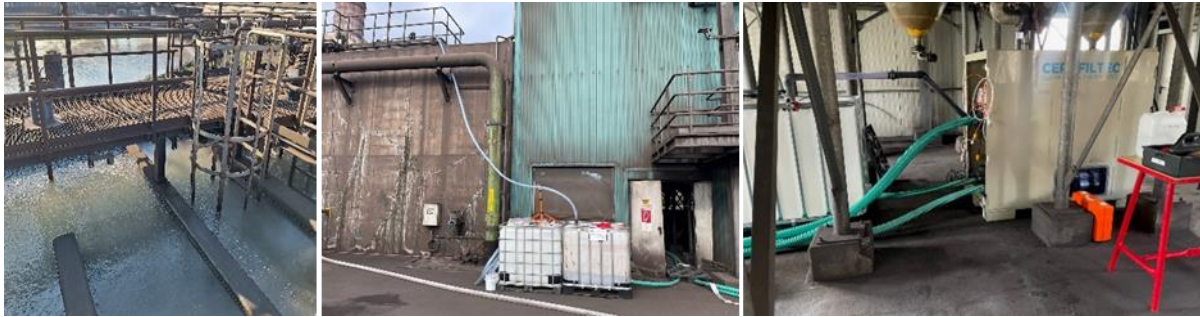
Figure 9 Field trial at effluent of the chemical treatment plant (CTP) of HKM (CTP (left), buffer and filtrate tanks in front of CTP (centre), ceramic flat sheet filtration at HKM (right)
