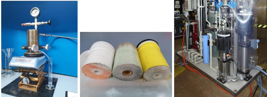
Figure 4 BFI-Lab test cell (left), exemplary membranes (mid), BFI technical scale nanofiltration unit (right)
